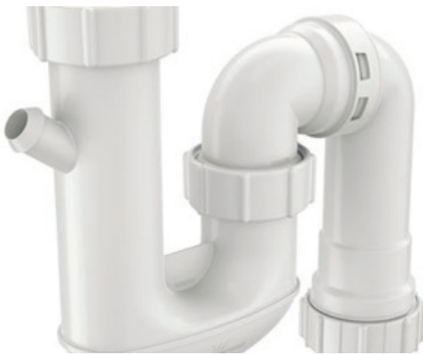
Figure 6: Typical waste trap from a sink with the dishwasher spigot.
