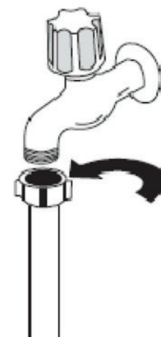
Figure 5: Connecting the supply hose to a ¾ inch tap.
