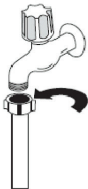
Figure 5- Connecting the supply hose to a \frac{3}{4} inch tap.
