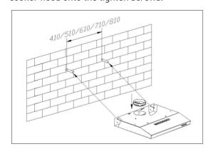
Fix the cooker hood with safety screw. The two safety vents are positioned on the back casing, with diameter of 6mm.
