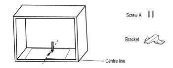
Remove the template and fix the mounting bracket in place with 2 x Screw A.
