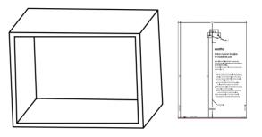
B) Make the marks on the bottom plane of the cabinet according to the "a" marks on the template.
