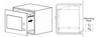
Open the door and fix the microwave into place using a screw, through the installation hole (indicated in the diagram below).
