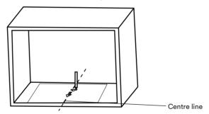
C) Remove the bottom cabinet template and fix the mounting plate with screws.
