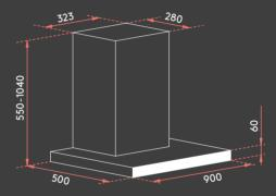
For safety and performance of your rangehood, adhere to the minimum and maximum distances from the rangehood base to the cooktop surface when positioning the rangehood for installation.
