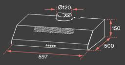
When positioning the rangehood for installation and use, we advise that the rangehood is mounted at a height of between 650mm–750mm above the cooking surface for safety and performance of your rangehood.
