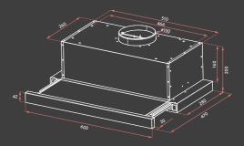
For safety and performance of your rangehood, adhere to the minimum and maximum distances from the rangehood base to the cooktop surface when positioning the rangehood for installation.
