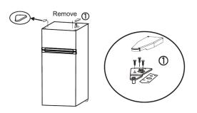
Remove the hinge cover. Unscrew and remove the top hinge.
