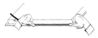
► Apply the sealing strip provided, around the edge of the appliance, and remove the protective covering.
