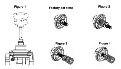
Note: Do not adjust the regulator valve body piece in the above procedure, otherwise it will affect the performance parameters set in the factory.
