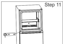
12. Install the F-door onto the middle hinge.
