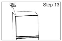
14. Mount the top left hinge cover to the top hinge, mount the hinge shaft cover to the top right of the refrigerator, mount the middle beam hole cover to the right side hole of the middle beam.
