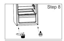
9. Remove the hinge bushing and door stop of the R-door and F-door with screw driver, and install them to the other side of the doors.
