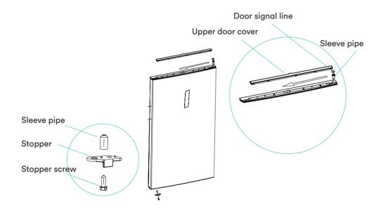
5. Take out the left top hinge and the left top hinge cover from the accessories package. Place the door on bottom hinge and mount top left hinge. Connect terminal 5 with terminal 1, then connect terminal 6 to the door switch. Connect terminal 2 with terminal 4.
