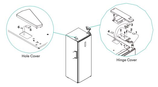
3. Dismantle the door and right bottom hinge assembly(hinge shaft&adjustable foot&hinge), disassemble the right bottom hinge assembly,and assemble the hinge shaft and adjustable foot on the other side of hinge, then assemble the whole hinge assembly on the other side of refrigerator.
